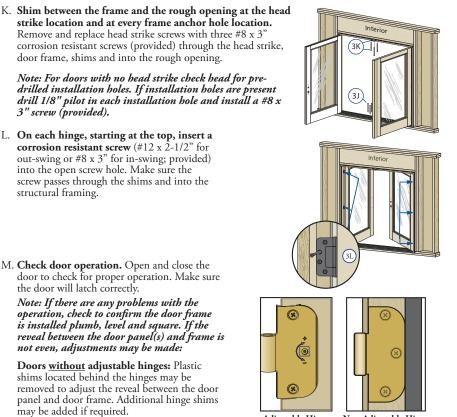
Adjustable Hinge Non-Adjustable Hinge
